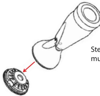
Step 3: Position the fixture on the mounting bracket. Note the 4 tabs on the inside of the fixture must drop into openings in mounting plate.
