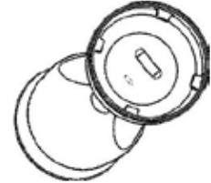
Step 4: While pushing fixture against mounting bracket, turn fixture clockwise until rigid resistance is encountered. Continue to turn past rigid resistance, and fixture will snap into place. Verify that the light is properly installed by rotating it counter clockwise about 1 full turn until the anti-rotation stop is encountered. The light should remain firmly installed. The anti-rotation stop will allow almost full rotation of the light, but will prevent the power wires from becoming twisted.
