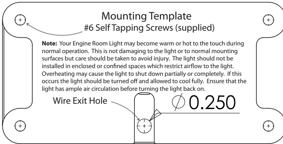
Light circuits should be protected with an appropriately sized fuse. Each light draws approximately 880mA at 12VDC and 440mA at 24VDC. Fuses on circuits with multiple lights should be sized accordingly.
