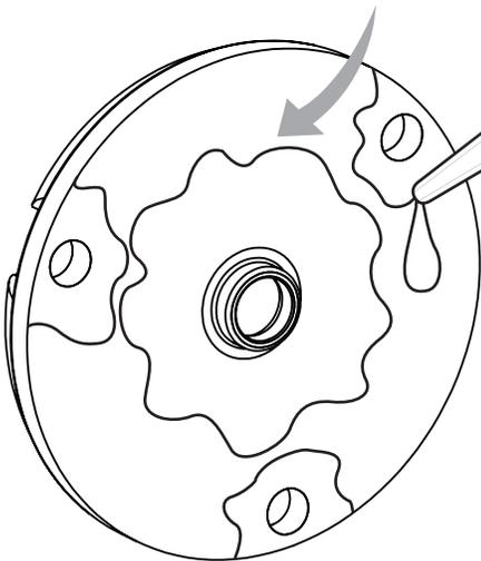
Lights may be painted, but ONLY with paints explicitly intended for aluminum substrates. Anti-fouling paints which do not explicitly state that they are safe for aluminum substrates can be damaging to the BayBlaze light, and should not be used on surfaces within 1" (2.5cm) of the light.
